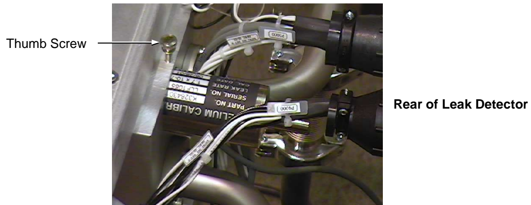
Figure 4-1 Location of the Calibrated Leak
